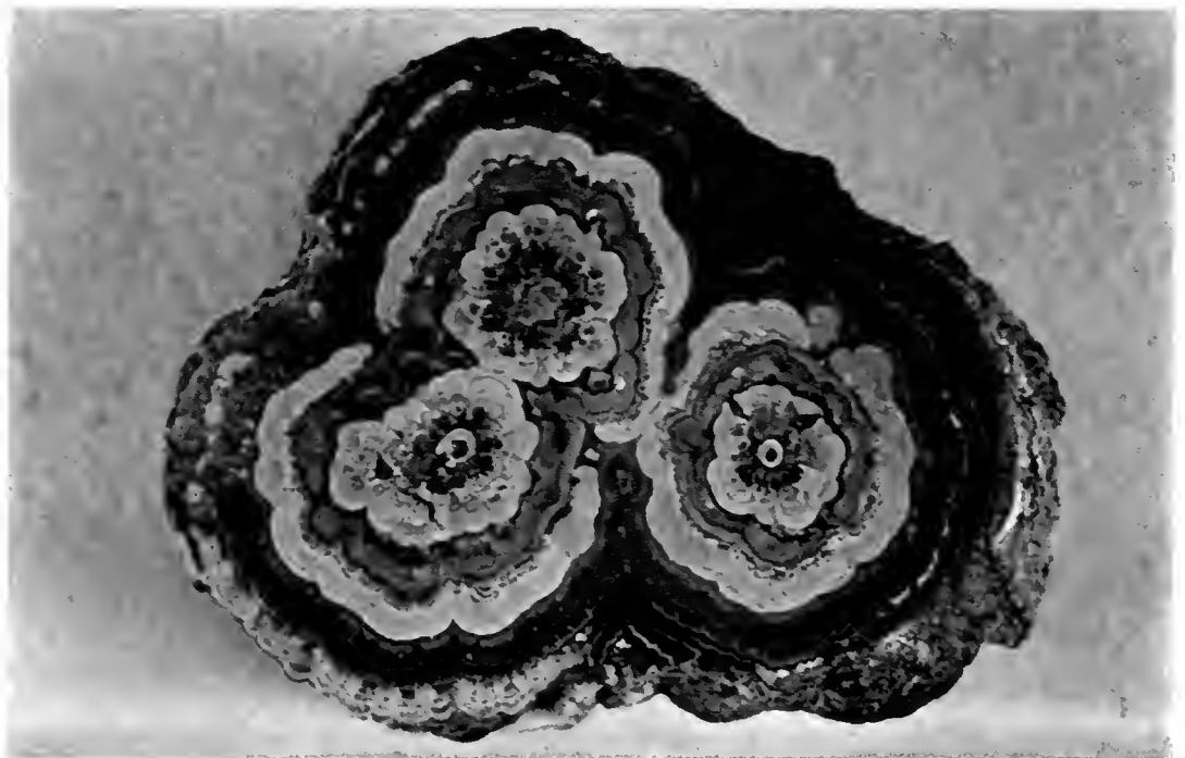
Cut and Polished Nodule of Copper Ore
